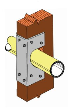
st pprox Approved stud shoes may be used when installed in accordance with the manufacturer's recommendations.
